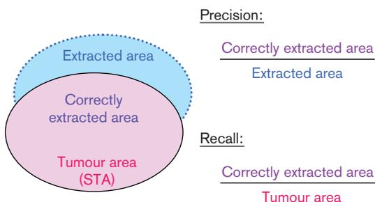
Tumour area and extracted area. Precision and recall are the performance indices of tumour area extraction. Precision reflects the accuracy of the extracted area and recall indicates how well the tumour area is extracted. STA, standard tumour area.
