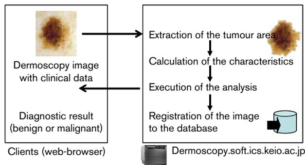
Protocol used by the web-based diagnostic system. When the server receives a dermoscopy image and clinical data, it performs tumour area extraction, calculation of the tumour characteristics and judgement based on an artificial neural network classifier. The server then registers the data to the database and finally sends back the diagnostic results to the client.
