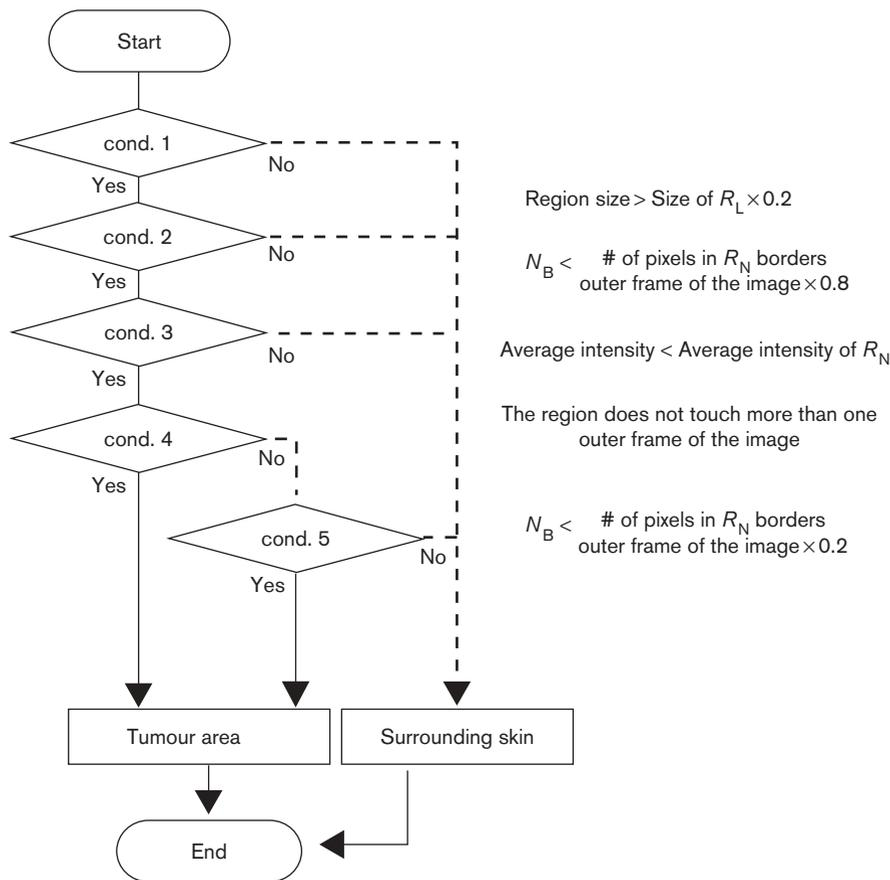
Flow chart of the tumour area selection phase of our tumour area extraction algorithm. Each segmented area is separated into tumour area and surrounding skin using this flow chart.  $N_B$ , number of pixel borders in the outer frame of the dermoscopy image;  $R_L$ , largest region;  $R_N$ , region bordering the external frame of the image with the longest boundary.
