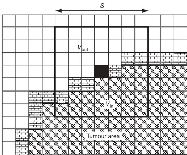
Concept of region-growing approach of our tumour area extraction algorithm. The temporarily decided tumour area was adjusted using a region-growing approach. For every border pixel (black pixel), the average intensities of the inside and outside of the tumour area,  $V_{in}$  and  $V_{out}$ , were calculated. In the corresponding equation, we regard the border to be ambiguous and treated the  $S \times S$  area as the tumour area.
