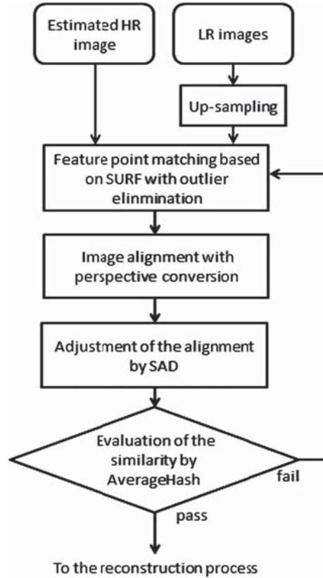
**Fig. 1.** Flow of the image alignment process.
