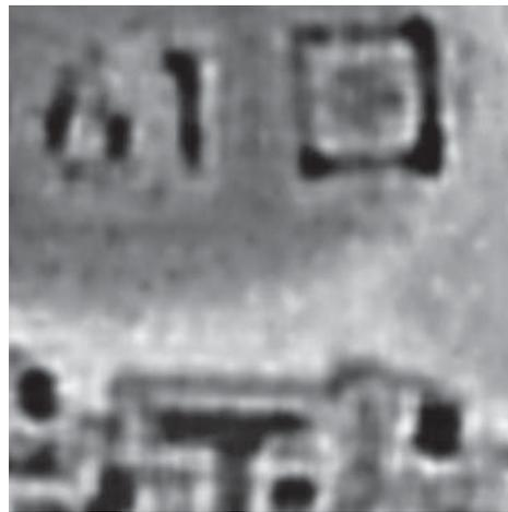
**Fig. 16.** Magnified view of super-resolution result of conventional method from 12 LR images.
