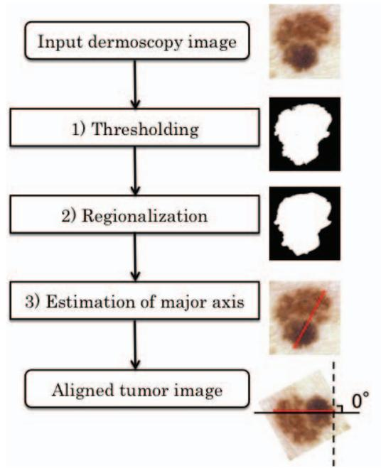
Fig. 1. Flowchart of the major axis alignment process.
