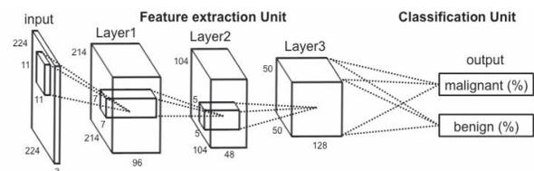
Fig. 2. Architecture of our simple CNN.
