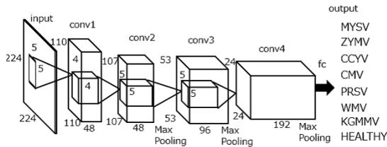
Figure 4. Proposed CNNs architecture
